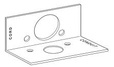
Replace cord/conduit plate and insert screws.
